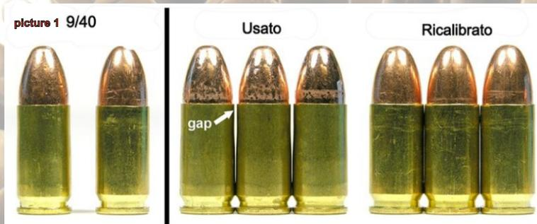
The use of recalibrated shells during the steps of reloading, makes the presses working with the least possible effort, avoiding then the formation of wears among the various linkages of the presses themselves, which as well known, are made of zamak, which is a very tender alloy aluminium and it is subject to rapid wears.
